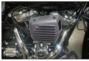
11. Install the  $K\&N^{\otimes}$  air filter and filter cover with provided bolts.
